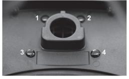
5. Remove the 4 black rivets from the underside of the visor carrier.
