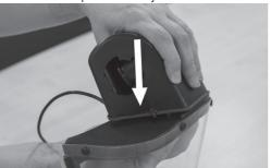
**3.** Now position the replacement motor on top of the peak plate and visor carrier then push home with the rivets (hold the motor down firmly whilst doing this).
