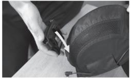
**6.** Rethread the wire through the sleeve and reconnect the plug to the battery.
