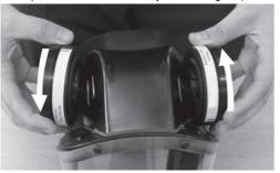
**5.** Reattach the filters by screwing them clockwise back into the two holes on either side.
