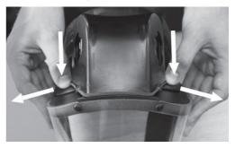
**4.** Now separate the visor from the cap. With the peak of the cap facing away from you, place your thumbs on either side of the cap's motor by the raised edges (as located by the two arrows), then press down and outwards, allowing the visor to slide away from the cap.
