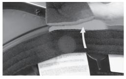
**4.** Make sure that you remove the visor's inner lining away from the velcro.
