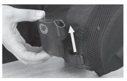
**3.** Remove the battery from the back of the cap by holding and sliding it upwards.
