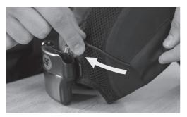
**5.** Rethread the wire through the sleeve on the side of the cap, then re-connect the wire to the battery.
