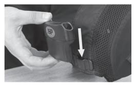
**4.** Replace the battery onto the back of the cap by holding and sliding it downwards.
