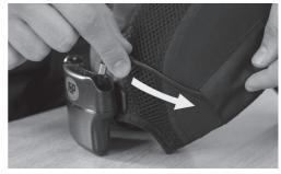
**2.** Disconnect the wire at the back of the cap and slide the cable through the sleeve on the side of the cap.
