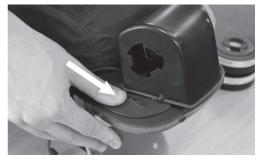
2. Holding the wire from the motor clear of the cap, slide the cap's peak between the motor and the visor back into position until you hear a 'click'.
