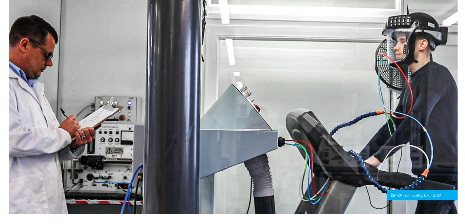
EN 12941 – Respiratory protective devices. Powered filtering devices incorporating a helmet or a hood. Requirements, testing, marking.
