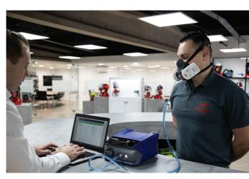
All methods require the test subject to carry out exercises to simulate movements made during work tasks.
